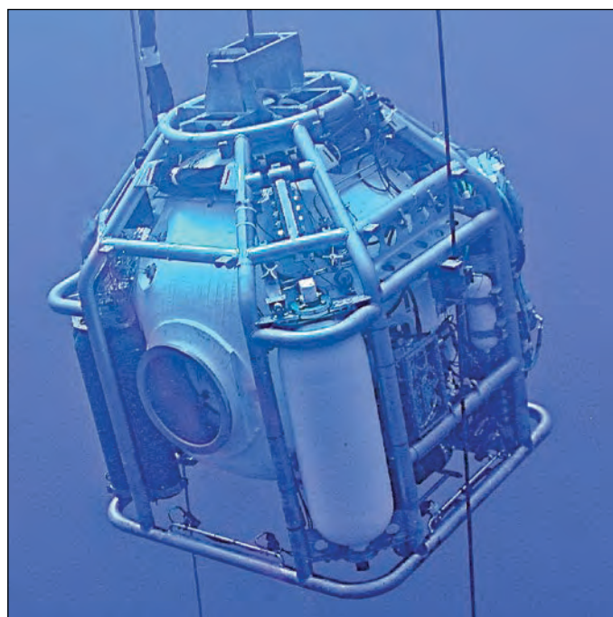
SAT FADS Dive Bell ascending thru the water Column after successful completion of the first 1000 fsw manned dive.
